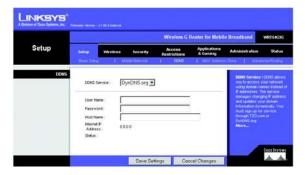
Figure 8-13: Setup Tab - DDNS (DynDNS.org)
